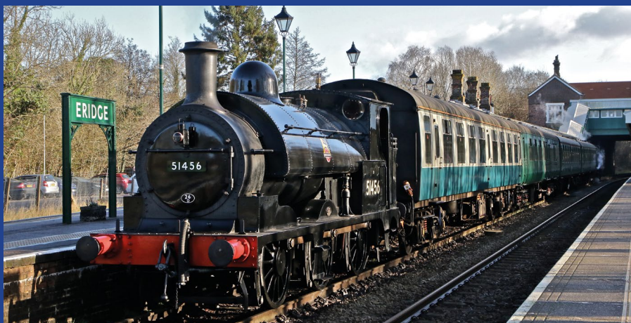
The Spa Valley Railway hired in ex-L&Y saddle tank 752 for their "Winter Steam Up" over the 8-9/1/22. The loco was built by Beyer, Peacock in 1881 as a tender engine then, when a crisis occurred and the L&Y found themselves short of shunting engines, 752 was rebuilt as a saddle tank to an Aspinall design at Horwich in 1896. Later on it became absorbed into the LNWR and later still into the LMS. In 1937 it was then sold into industrial use to the Blainscough Colliery Railway. It now appears in BR black and carries the number 51456, the next number in sequence, although it was never on the books of British Railways. It is seen here at Eridge on 9/1/22.
