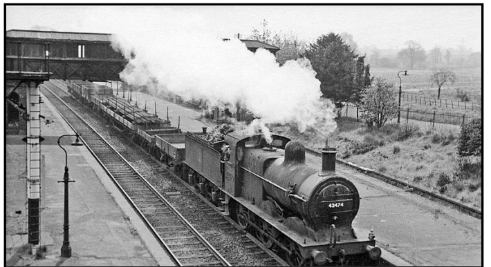
▲ “3F” 0-6-0 No. 43474 heads South past Amphill. Over-length load on Bogie bolster. Single bolster as match truck. Class K “pick-up goods” headcode. Makes one feel old. Bill Davies collection.
